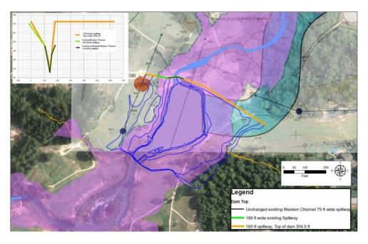
The Halff Flood plain impacts study, overlaid on GolfScapes Inc. proposal to multiple overflow routes for the 100 year storm (shown in light blue). This is a mid design plan, as the two firms collaborated back and forth to reach a final design that met requirements. The 18th and 16th holes shown below.
