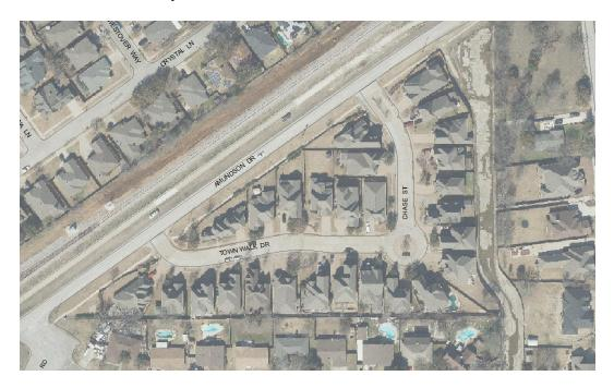
The intersection of Town Walk Drive and Chase Street includes a circular landscaped island which channelizes traffic flow around that feature. As residential roadways on the City's Transportation Plan (formerly Master Thoroughfare Plan) both streets are 30-feet in width from face of curb to face of curb. With the 30-foot width, there is insufficient room to support both unobstructed two-way traffic and extensive on-street parking on both
