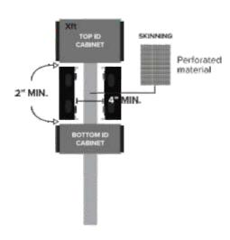
2" MIN. space required on top and bottom of the display required to meet warranty. To increase convection, the sides of the display can be left open or covered with a perforated material.
