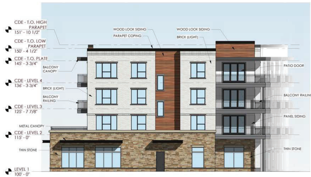
3 BUILDING E - SOUTH ELEVATION SCALE: 1" = 10'-0"
