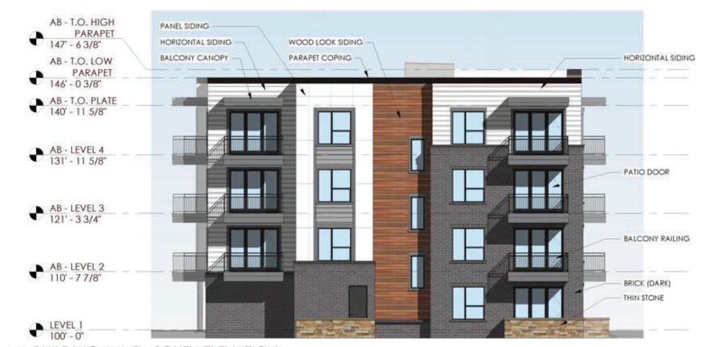
3 BUILDING A & B - SOUTH ELEVATION SCALE: 1" = 10'-0"
