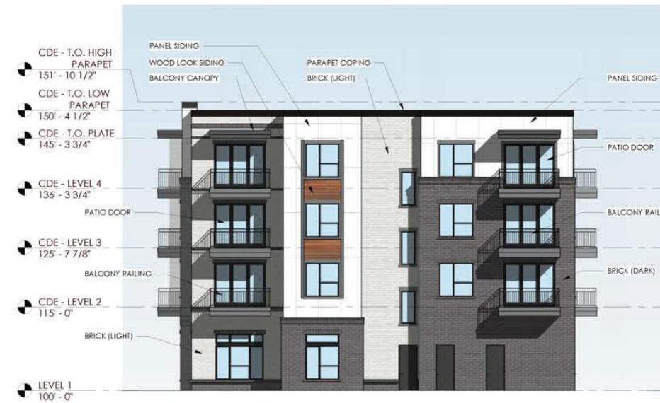
2 BUILDING E - NORTH ELEVATION SCALE: 1" = 10'-0"
