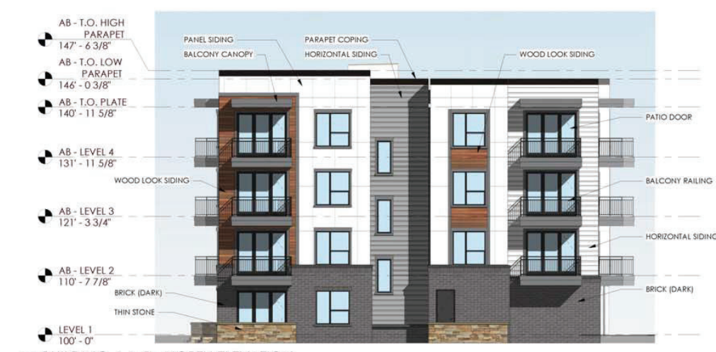
2 BUILDING A & B - NORTH ELEVATION SCALE: 1" = 10'-0"
