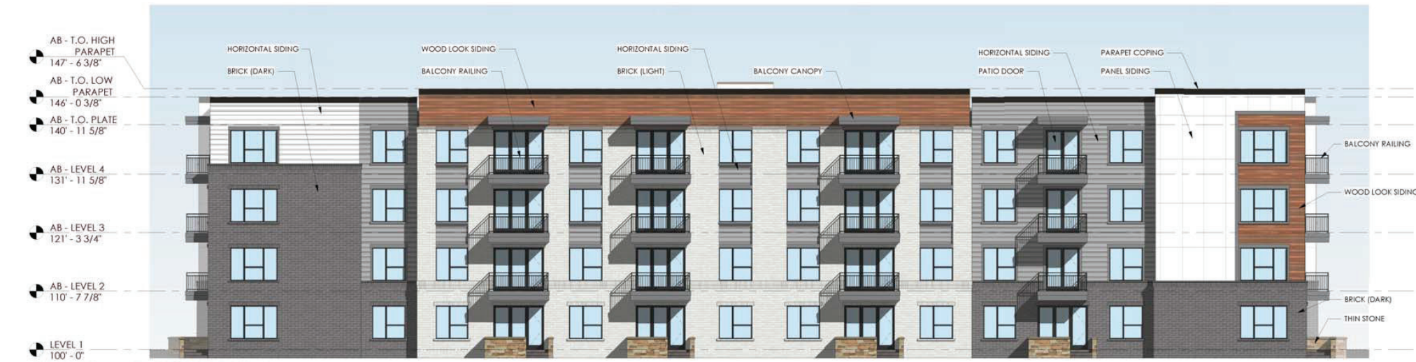
1 BUILDING A & B - EAST ELEVATION SCALE: 1" = 10'-0"
