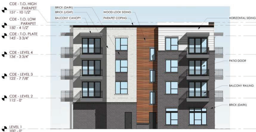
3 BUILDING C & D - SOUTH ELEVATION SCALE: 1" = 10'-0"
