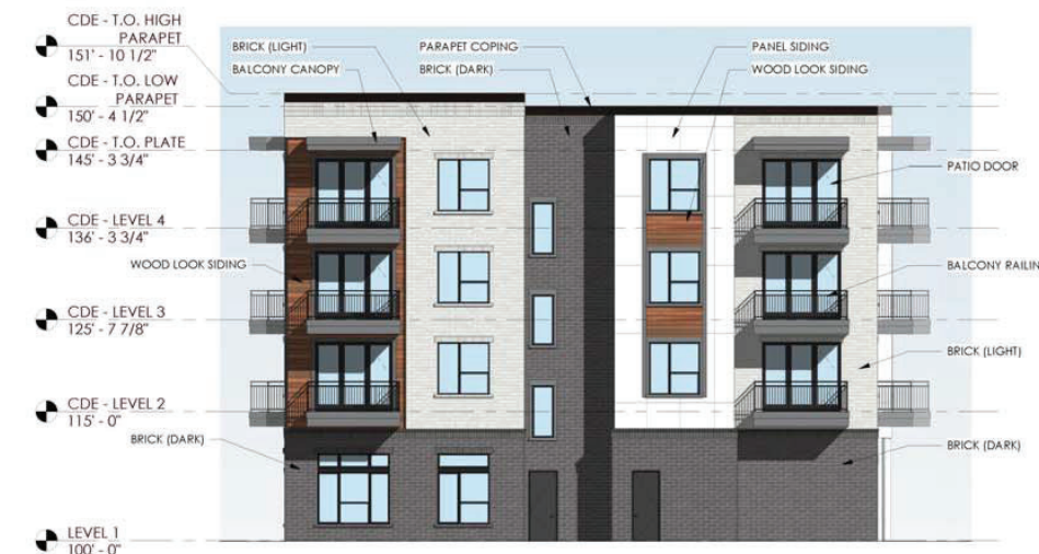
2 BUILDING C & D - NORTH ELEVATION SCALE: 1" = 10'-0"
