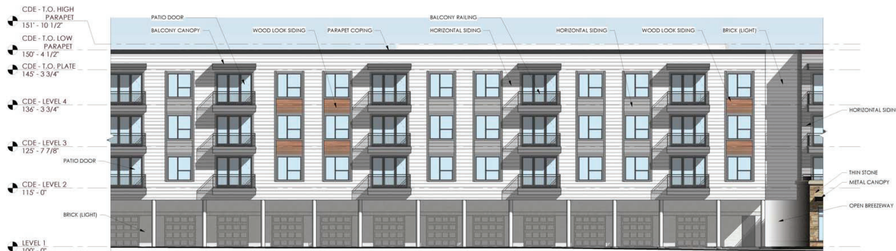
2 BUILDING E - WEST ELEVATION B SCALE: 1" = 10'-0"
