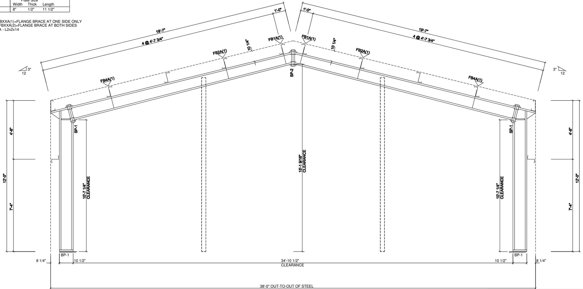
RIGID FRAME ELEVATION: FRAME LINE 1 3
