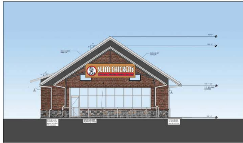
01 SOUTH ELEVATION SCALE: 1/4"=1'-0"
