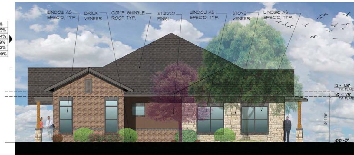
04 VILLA - SIDE EXTERIOR ELEVATIONS SCALE: 3/16" = 1'-0" (2-UNIT VILLA)
