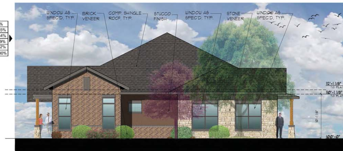
04 VILLA - SIDE EXTERIOR ELEVATIONS SCALE 3/8" = 1'-0" (2-UNIT VILLA)
