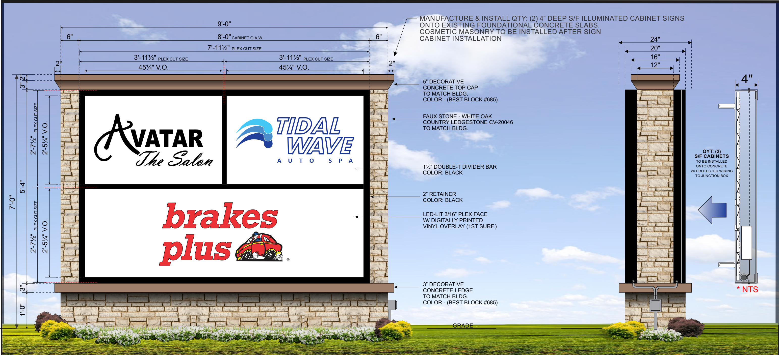
D/F MONUMENT SIGN W/ ILLUMINATED PLEX FACE CABINETS QTY: (2) LED ILLUMINATED CABINETS REQUIRED Scale: 3/4" = 1'-0" STONE/MASONRY BY OTHERS
