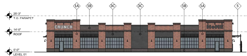
7 NORTH ELEVATION - BUILDING 7 (RETAIL) SCALE: 1/16" = 1'-0"
