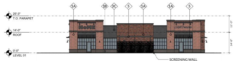
6 WEST ELEVATION - BUILDING 7 (RETAIL) SCALE: 1/16" = 1'-0"
