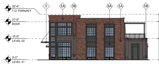
4 SOUTH ELEVATION - BUILDING 5 (CLUBHOUSE) SCALE: 1/16" = 1'-0"
