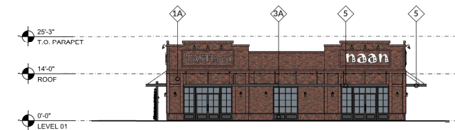
3 NORTH ELEVATION - BUILDING 6 (RETAIL) SCALE: 1/16" = 1'-0"
