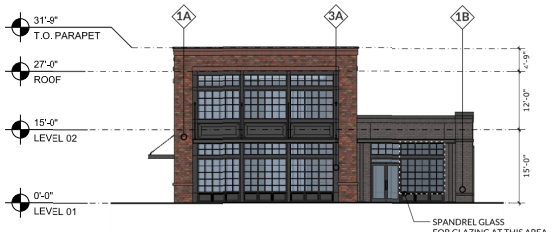
8 SOUTH ELEVATION - BUILDING 4 (FITNESS) SCALE: 1/16" = 1'-0"
