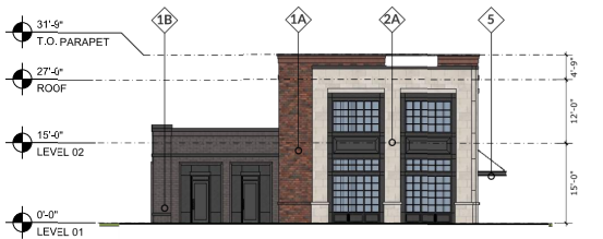
7 NORTH ELEVATION - BUILDING 4 (FITNESS) SCALE: 1/16" = 1'-0"
