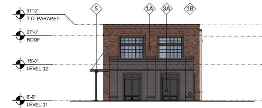
5 EAST ELEVATION - BUILDING 4 (FITNESS) SCALE: 1/16" = 1'-0"
