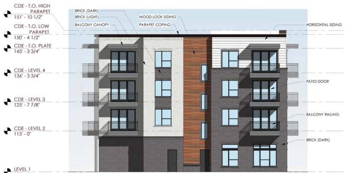
3 BUILDING C & D - SOUTH ELEVATION SCALE: 1" = 10'-0"
