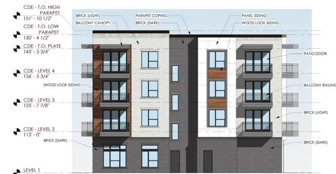
2 BUILDING C & D - NORTH ELEVATION SCALE: 1" = 10'-0"
