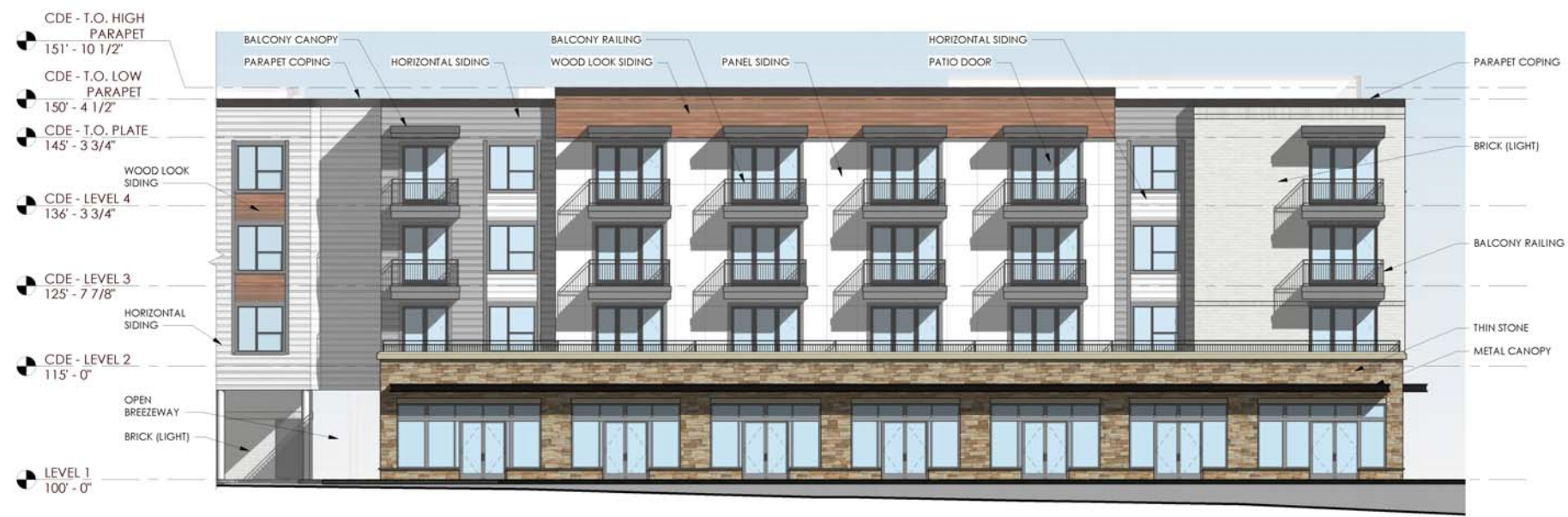
3 BUILDING E - WEST ELEVATION C SCALE: 1" = 10'-0"
