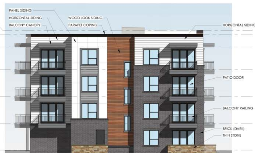
3 BUILDING A & B - SOUTH ELEVATION SCALE: 1" = 10'-0"
