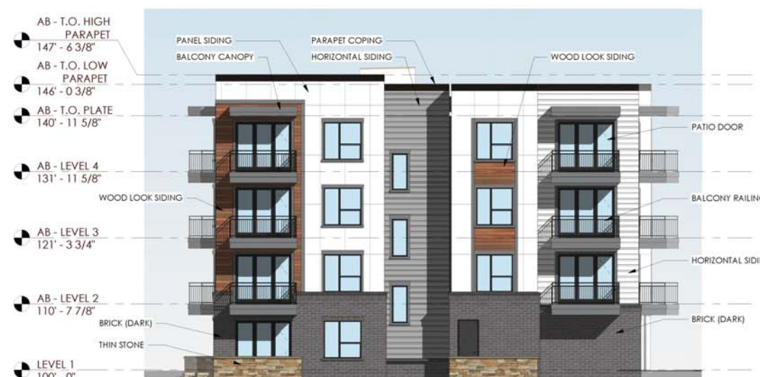
2 BUILDING A & B - NORTH ELEVATION SCALE: 1" = 10'-0"
