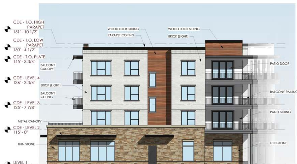
3 BUILDING E - SOUTH ELEVATION
