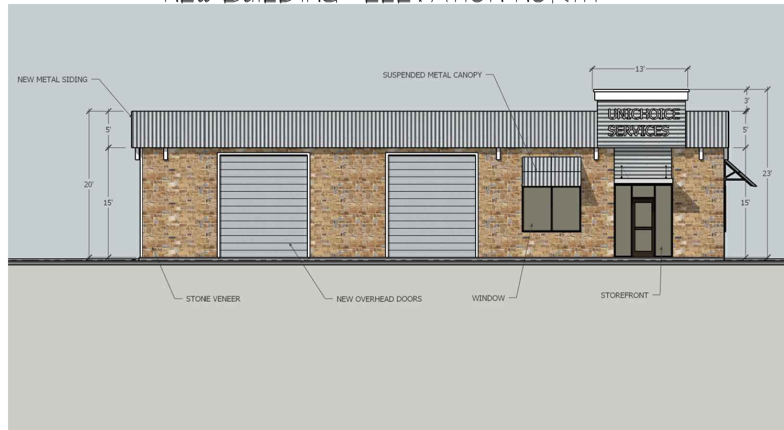
NEW BUILDING - ELEVATION SOUTH
