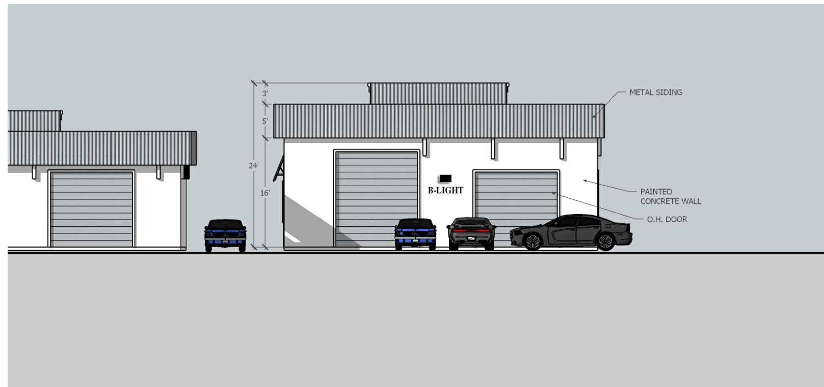
SPEARS CORPORATION BUILDING -ELEVATION EAST
