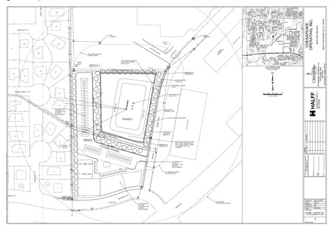
2012 gas well pad site Special Use Permit exhibit demonstrating developable area outside a 150-foot no-build easement
