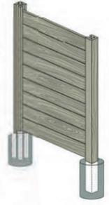
Superior Ledgestone™ will have a new and improved tongue and groove panel interlocks, which may result in the appearance of grooves between panels.
